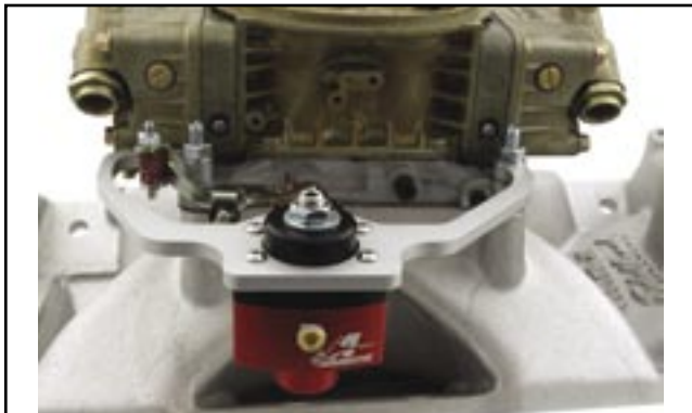
ALL54280 Bracket - Shown With Aeromotive Regulator
