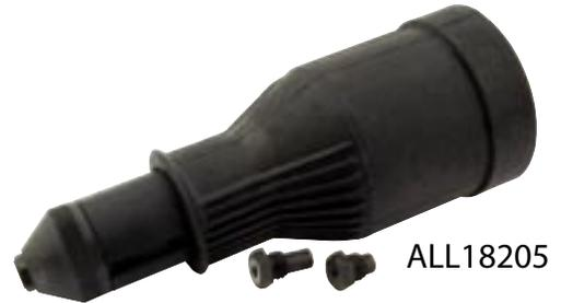
**INSTALLATION:** Always use a reversible drill and set to drill position. Experiment with high and low speeds to achieve best results. Open the drill chuck and insert the shank of ALL18205 (FIG. 1). Tighten the chuck securely and cover with "telescopic" protective sleeve. Three nosepieces are included (use the same nosepiece for 3/32" & 1/8" diameter rivets). Use the proper size nosepiece for the rivet being installed.
